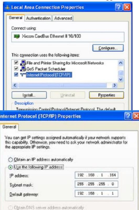
When logger working in "Obtain and IP address automatically" mode, and the led-ETHERNET flash slowly. The IP address of the logger is "192.168.1.250" always, you need to change your PC set-. Subnet as "192.168.1.\*", and the Default gateway must be "192.168.1.1"
